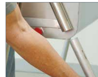
Slide frame legs all the way up into the fixtures on the side of the tank with the lid closed.
